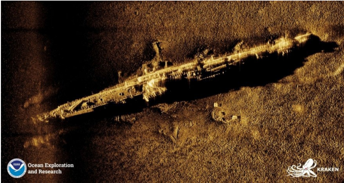
Synthetic aperture sonar imagery of a German submarine
