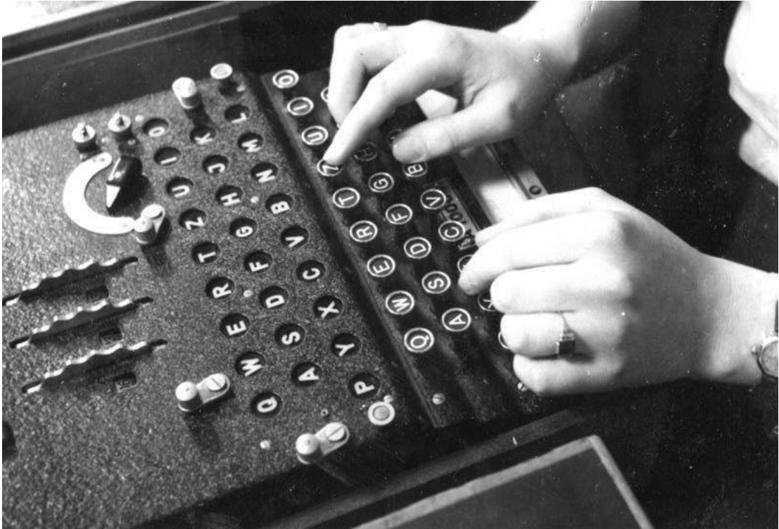
A German Enigma Machine in Use Source: Bundesarchiv_Bild_183-2007-0705-502, Chiffriermaschine 'Enigma'
